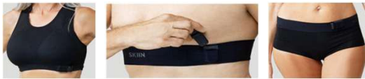
Figure 1: Images of garments (SKIIN) with sensor woven into the textile with software to monitor and transmit information to a data repository for analysis and monitoring. Bra (left); chest band (centre); and underwear (right).
